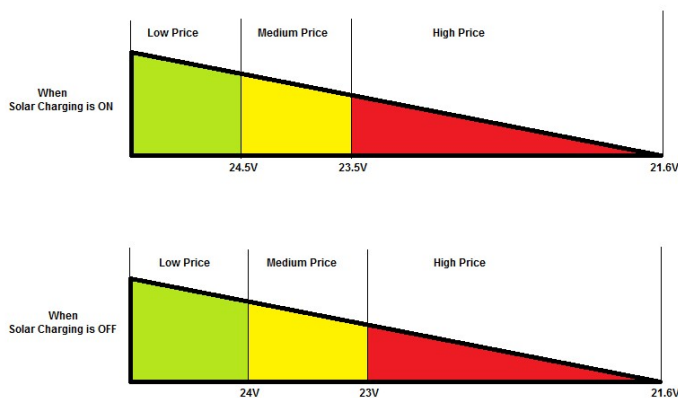
Figure 3.2. Electricity price levels defined by the battery bank voltage. Figure: EmSys Electronics
