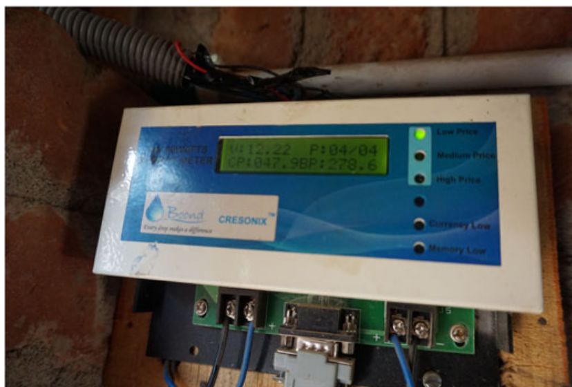
Figure 2. Energy meter of a pico-grid is an example of a frugal solar component.
