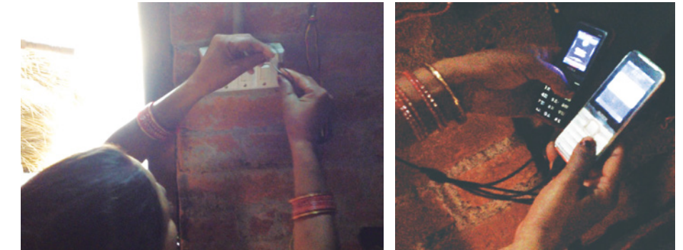
FIGURE 19 A participant disconnects phone charging cables from the Boond system and reconnects them to the SHS battery to charge the family's two mobile phones.
